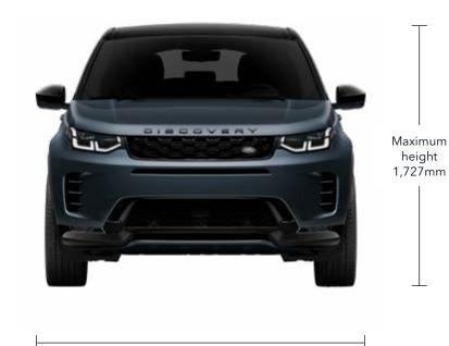
Width 2,069mm mirrors folded Width 2,173mm mirrors out
